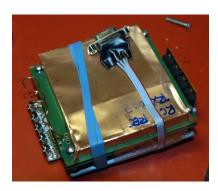
Pins 2, 3, and 5 are standard RS232 connections, pin 5 common (GND) for both data and power. Pin 9 is used for 12VDC power in. RS232 can connect directly to a PC with a standard cable (pin 2 to 3, crossover, in each direction). 12VDC must be provided to pin 5 (GND) and pin 9 (+V). Avoid routing 12V to the connected PC, do not use pin 9 on the connection to the PC.
