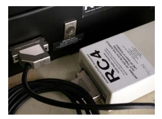
Connect a DMX source to the DMX input on the transmitter. The RC4-TXD-series DMX input is not terminated. A terminated cable or in-line termination connector must be used if termination is required (i.e. the transmitter is at the end of the DMX line). In general, a 120-ohm resistor between pins 2 and 3 of a DMX connector will provide adequate termination.
