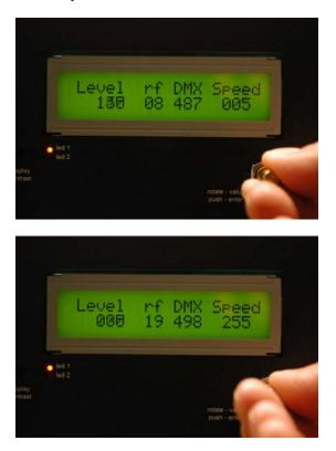
Select which channels will be part of the chase by pressing the **Manual Channel Test** key and making changes there. You can then return to the chase by pressing **Channel Chase Test**. It is not necessary to press **Exit** between these modes.
