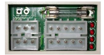
In some cases, the 6-pin connector can be used for high-power battery input, while the 10-pin connector can be used just for outputs. If all pins of both connectors are used, eight wires are available for both power in and dimmer out. This results in symmetrical current carrying capacity on both sides of the dimmers.
