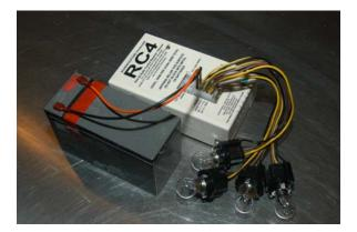
Radio and dimmer control electronics will not operate properly with less than 10V of incoming power. This voltage must be maintained under load. Choose appropriately sized batteries and keep them charged.
