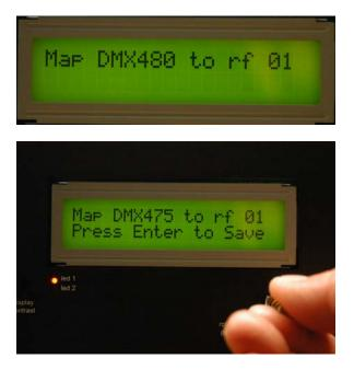
Similar to *Watch Channels* mode, the rotary control will select CV inputs above DMX 512 and below DMX 1. This makes it easy to assign any of the 8 available CV inputs to any rf dimmer channel, with the rotary control providing access to 520 sources (512 DMX channels and 8 CV channels).
