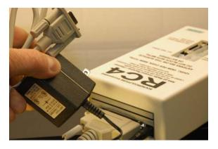
Do not attempt to change system settings while powering the receiver from the 10-pin RC4 power connection. This powers both the radio board and the dimmer logic board, and does not leave the radio board available for data on the rear 25-pin port.
