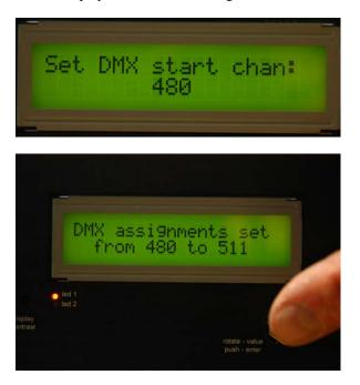
When first entering this mode, the DMX channel currently being watched is displayed as the starting channel. You may change this by turning the rotary control.
