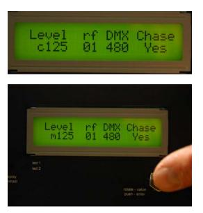
The Chase parameter is used by the Channel Chase Test function described below. It is toggled between Yes and No for the currently displayed rf channel by pressing the **Select/Enter** key.
