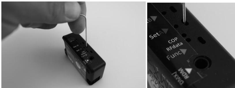
**Pressing SetA on an RC4 Series 3 DMX2dim.** The DimA indicator is behind the round hole. The button is behind the slotted hole. With a DMX channel set higher than 20%, press the SetA button and the DimA indicator will come on. Dimmer A is now assigned to that channel. It remembers this setting until you change it by pressing the button again.
