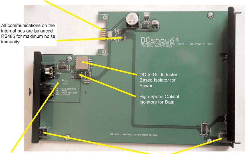
USITT DMX512A compliant data inputs, optically isolated and fully floated, safe to 5000V differential.
