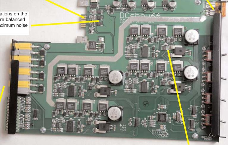
Anderson connectors for motor power outputs. Removeable screw-terminal block for limit switch inputs. Each motor driver has two limit switch inputs, for cw and ccw limiting.
