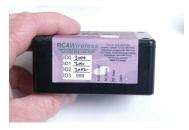
The **RF Active** indicator will light continuously after power-up, while radio channels are being scanned. When a clear channel is located and transmission has begun, this indicator will blink slowly and steadily. *In normal operation, this led should be blinking.*
